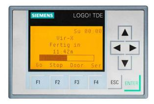
Disinfection should not be interrupted. In emergencies, disinfection can be interrupted via the F2 key. Depending on the ozone concentration, however, the door can only be opened after a certain time. The display informs you of the current status of the system.
